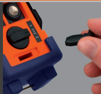
radiomatic® iLOG for quick activation of a spare transmitter.
